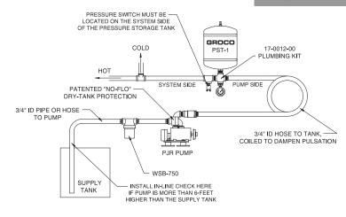
PLUMBING: Fasten 17-0012-00 plumbing kit onto the PST (pressure storage tank) with the pressure switch on the system-side of the PST and the hose barb on the pump-side of the PST as shown above. To aid in initial priming, pour water into the pump inlet before connecting hoses to the pump. Plumbing between the pump and the PST must be 3/4" ID heavily reinforced hose, and must be free of valves, filters, or any other device. Plumbing after the PST may be reduced.
