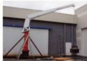
Cranes are proof tested to 110% of capacity
