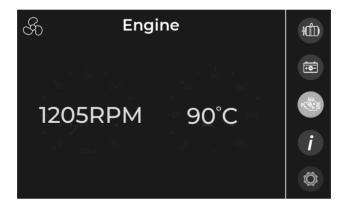
The system indicates if the engine is in or out of gear. The gear status is displayed at the top left with a propeller symbol.\*
