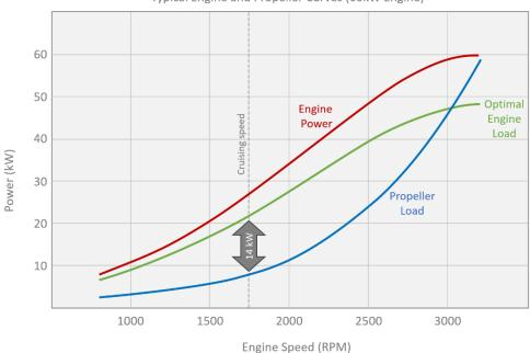
Typical Engine and Propeller Curves (60kW Engine)
