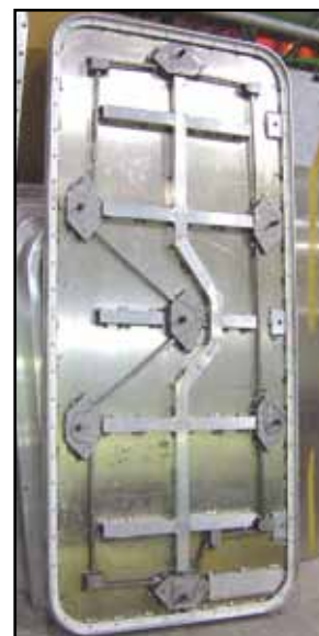
Chain-drive, Stiffeners, Interior panel with inspection plate at left in photo
