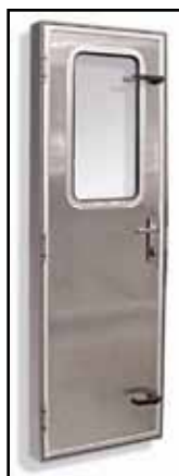
Steel coaming, Mitered corners, Two dogs, lockset, Upper half large window
