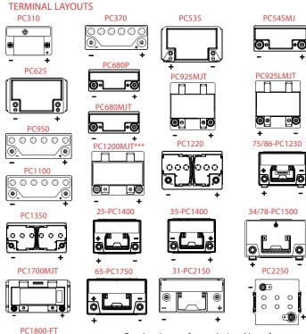
Drawing sizes are for terminal position reference only; diagrams are not proportionate to each other. \*\*\*Optional Reversed Polarity (L) available. Non-stock item
