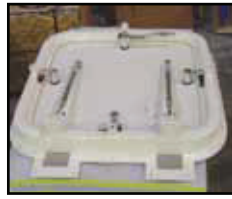
Deep gutter, Gas springs on coaming, Closed
