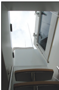
Ladderwell hatch, Proud coaming, Open, Interior
