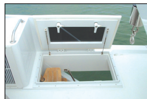
Ladderwell hatch, Proud coaming, Open, Exterior
