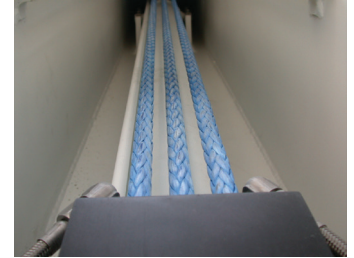
Whisper quiet linear winches use composite rope which is quieter and stronger than steel cable
