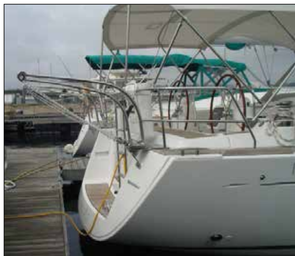
2007 Beneteau 49 with Custom Davit Mounting Brackets
