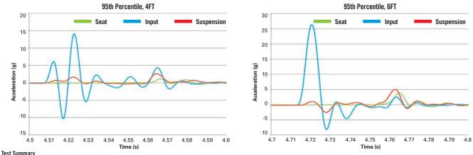
• Shock experienced by a 95th percentile occupant (225lbs/103kg) was reduced from 26G to 3.8G - an 85% reduction - in laboratory testing. Weight adjust range was set to the maximum.
