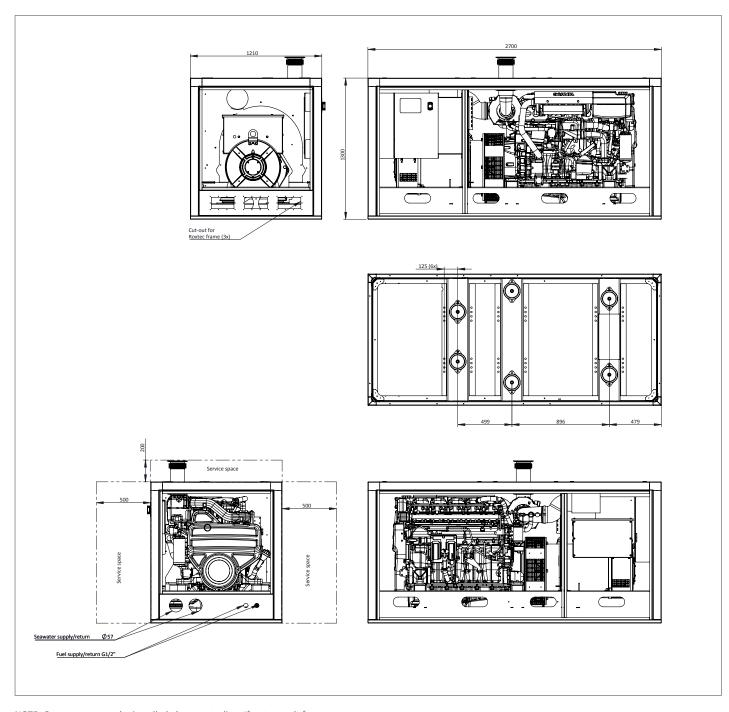
NOTE: Generator sets to be installed above waterline. If not consult factory.
