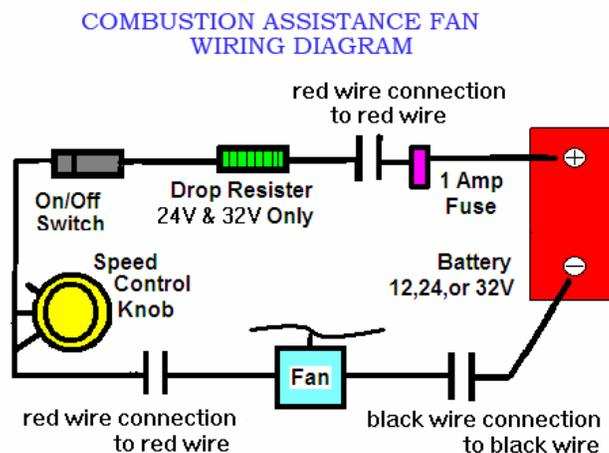
During start up, operating at higher settings or during windy conditions, you want to use the combustion assist fan on your heater to artificially boost the draft. Your heater should operate without the use of the fan on lower temperature settings. Some heater installations with only the minimum flue heights or with flue elbows that inhibit the draft may need the use of the fan more often.
