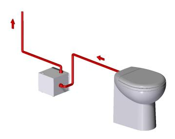
In the case of **connection to the Planus aspirator box**, you will have to connect the inlet of this box to the connection on the back of the toilet ( $\emptyset$  25 mm). Furthermore, the exhaust of the vacuum box must be connected to the outside of the hull.
