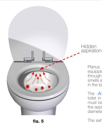
Planus nautical toilets in AirEx version are equipped with an aspiration system, invisible, through which contaminated aerosol and unpleasant smells are extracted (fig. 5), preventing their spread in the bathroom.
